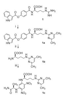
**Figure 2.** Derivatization of compound 1 for Marfey analysis: (i) H<sub>2</sub>O (25  $\mu$ L), EtOH (50  $\mu$ L), triethylamine (25  $\mu$ L), and acetylacetone (50 $\mu$ L), 110 °C, 4 h; (ii) 2 N HCl, 110 °C, 6 h; (iii) FDAA (1-fluoro-2,4-dinitrophenyl-5-L-alanine amide), 40 °C, 2 h.
