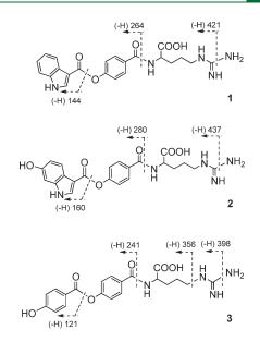
Figure 3. Prominent fragmentations of the  $[M + H]^+$  ions of compounds 1-3 in FAB-CID tandem mass spectrometry.
